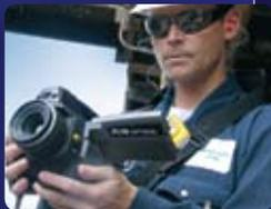
FLIR's GF-306 optical gas imaging camera can locate SF6 leaking from energized equipment and help you comply with the new EPA Greenhouse Gas Reporting Rule, Subpart DD, by reducing overall SF6 emissions before the March, 2011 report deadline.
