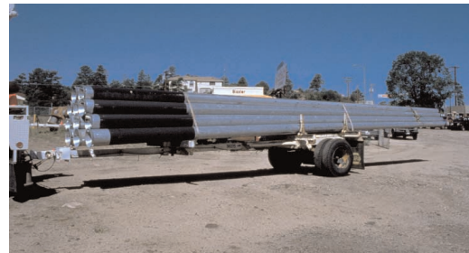
Because steel poles are lighter than wood, they are easier to transport and carry to job sites.
