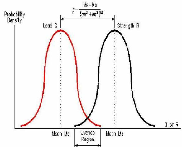
Fig. 1. Random nature of structural strength and variability of storm loadings.
