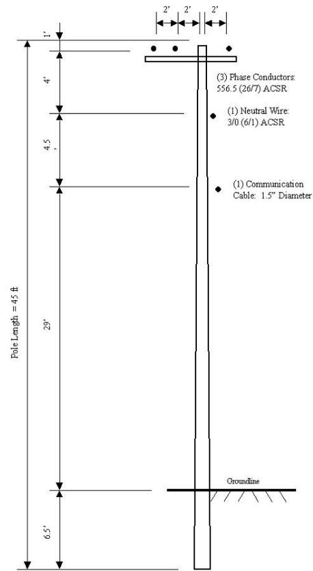
Fig. 2. Sample Distribution Pole Design Example.
